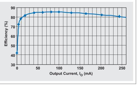
the low- $R_{\rm DS(on)}$  internal switches and the choice of switching frequency provide optimal supply efficiency. Figure 2 shows efficiency data for a 12-V output when a Li-ion battery with a typical 3.6-V source voltage is used.
