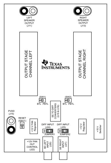
Figure 2. Physical Structure for the TAS53630PHDEVM (Approximate Layout)
