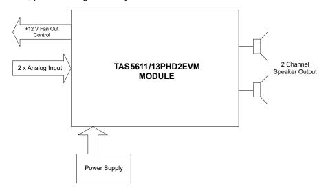
Figure 1. Integrated PurePath™ Digital Amplifier System
