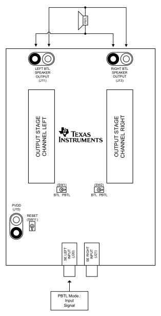
Figure 3. Figure 3. PBTL Mode Configuration
