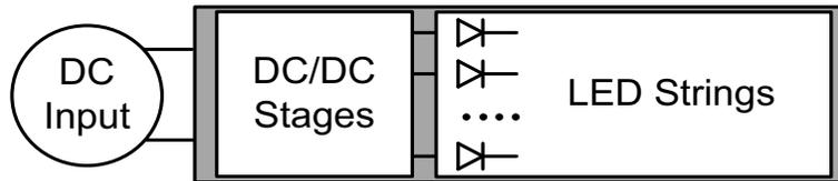
**Figure 2. Block Diagram for an LED Lighting Application**
