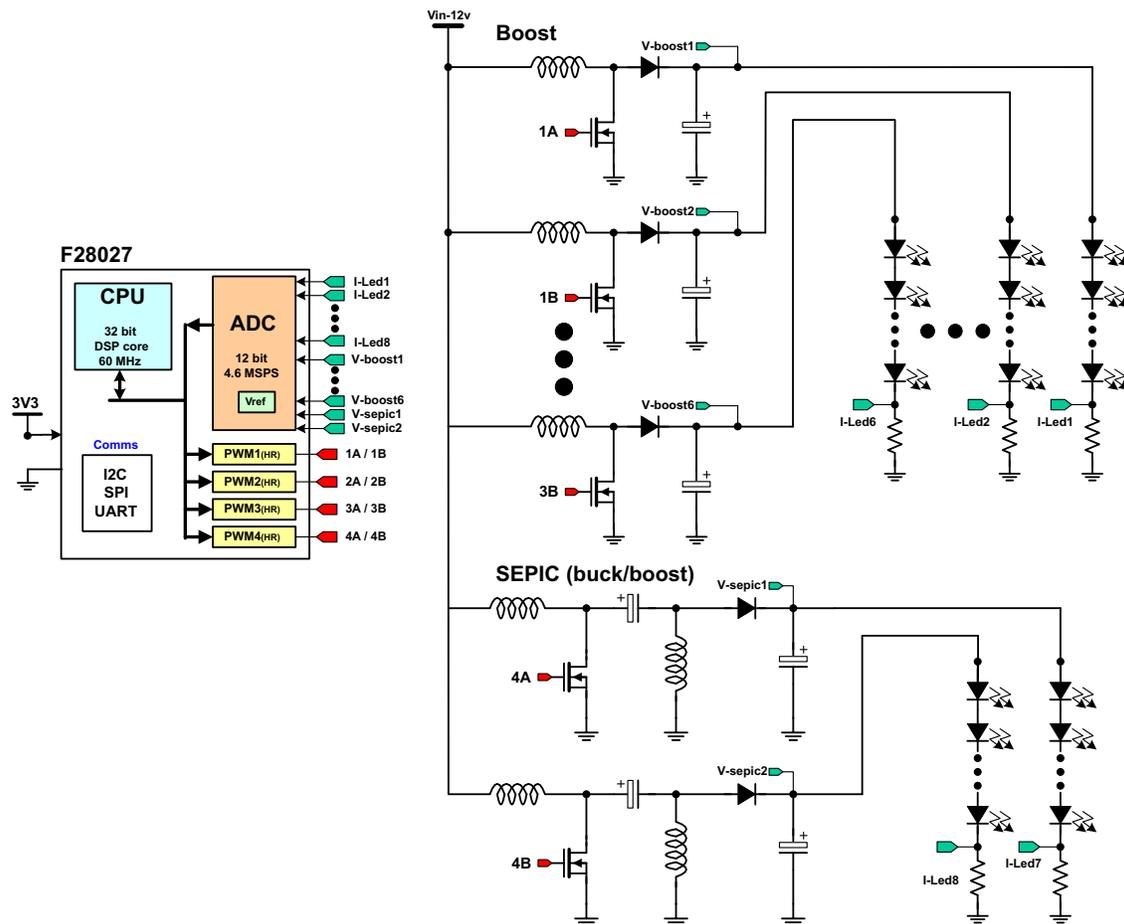
Figure 4. Multi-DC/DC Color LED Kit Circuit Diagram
