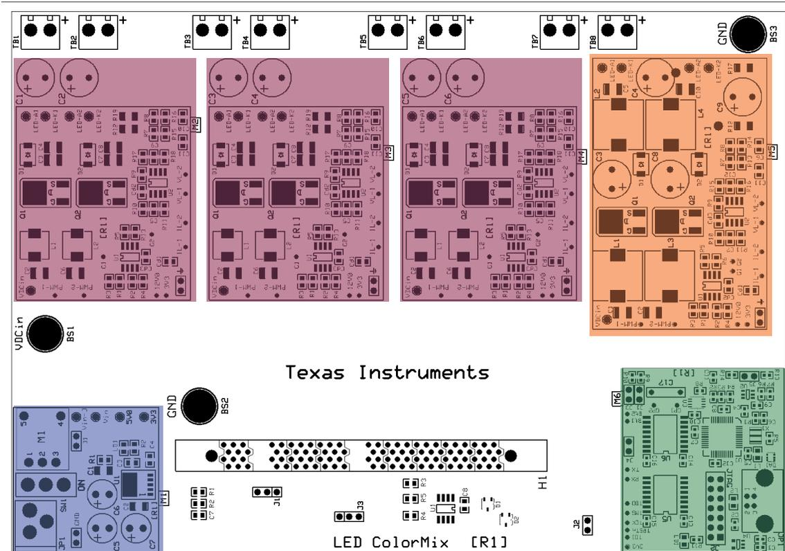
**Figure 3. Multi-DC/DC Color LED Board Macro Block Locations**
