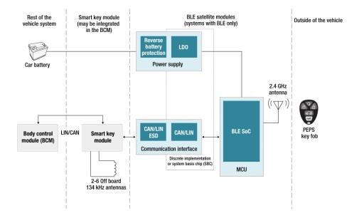
Figure 2. : Automotive PEPS System Block Diagram
