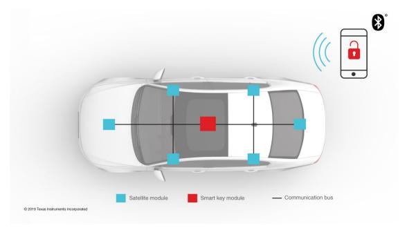
Figure 1. Bluetooth Low Energy PEPS Architecture in a Car
