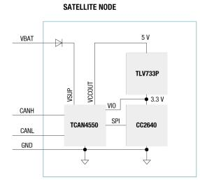
Figure 3. : The TCAN4550-Q1 Makes It Easy to Add CAN Communication to the Satellite Node
