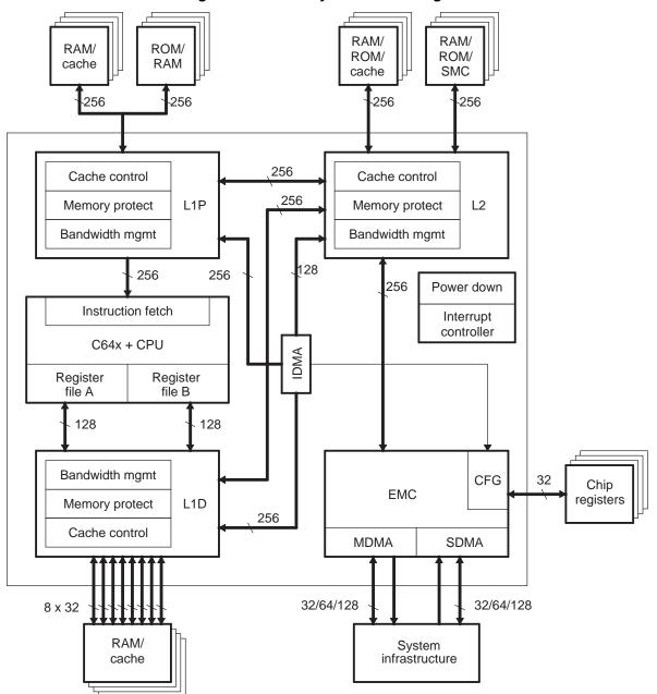
Figure 1. DSP Subsystem Block Diagram
