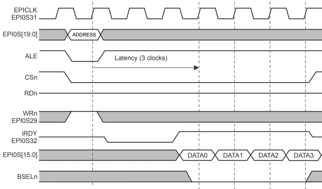
Figure 11-8. PSRAM Burst Write
