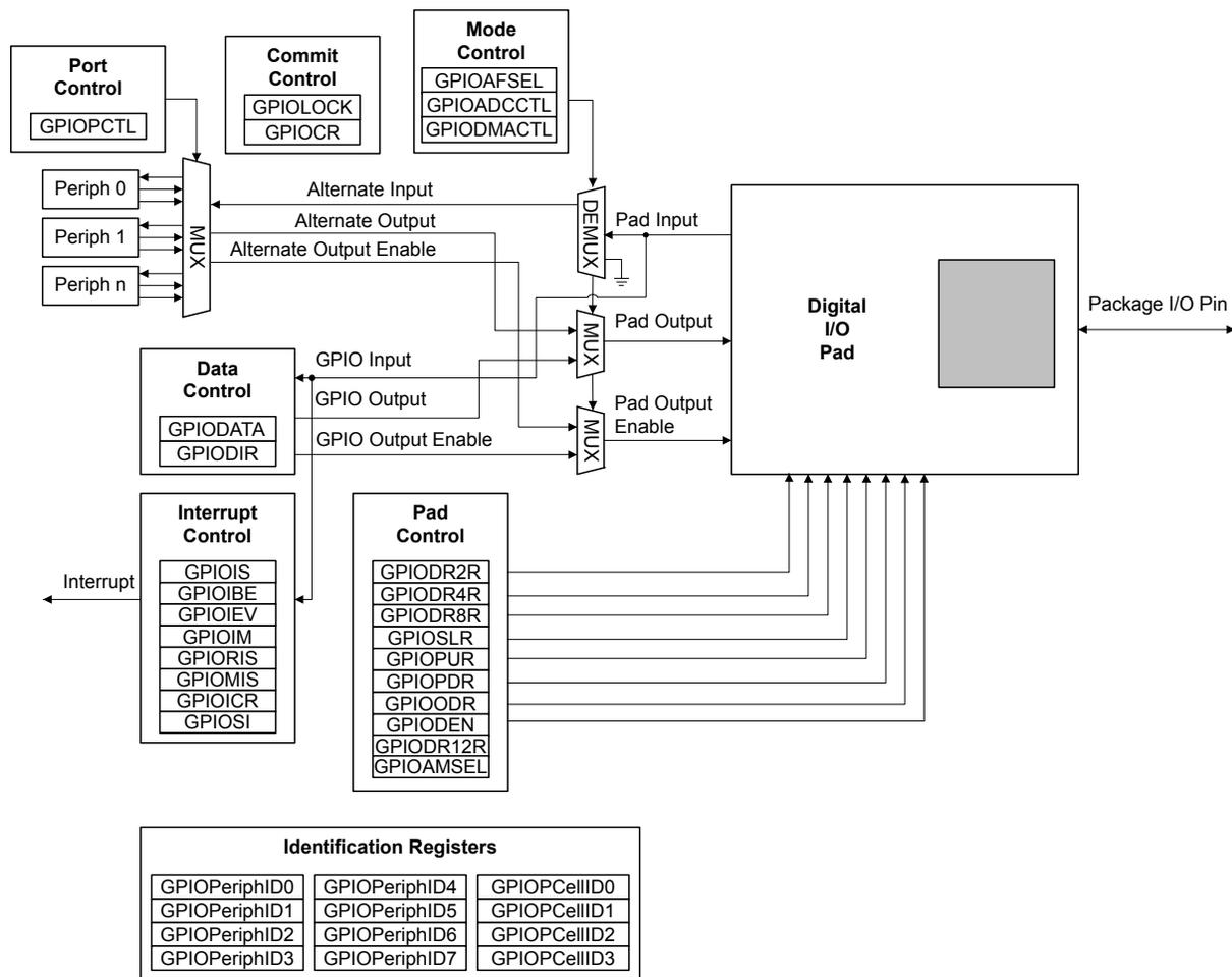
Figure 10-2. Analog/Digital I/O Pads
