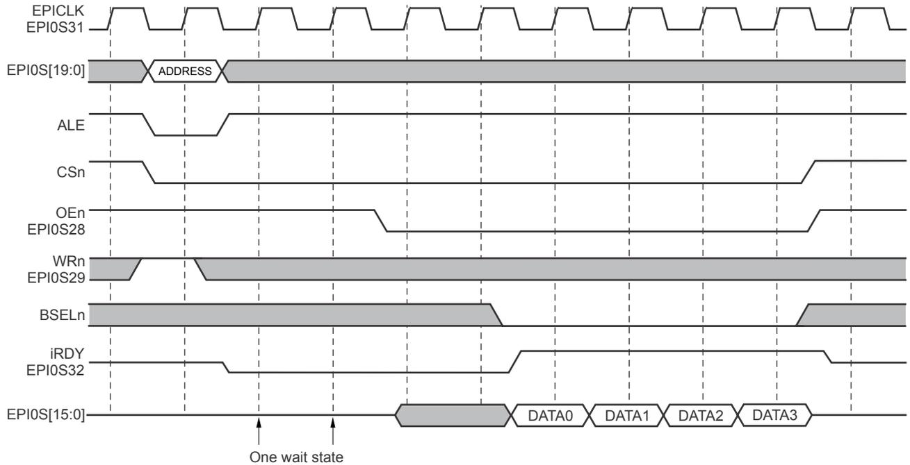
**Figure 11-10. Write Delay During Refresh Event**
