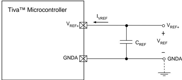
Figure 27-29. ADC Input Equivalency
