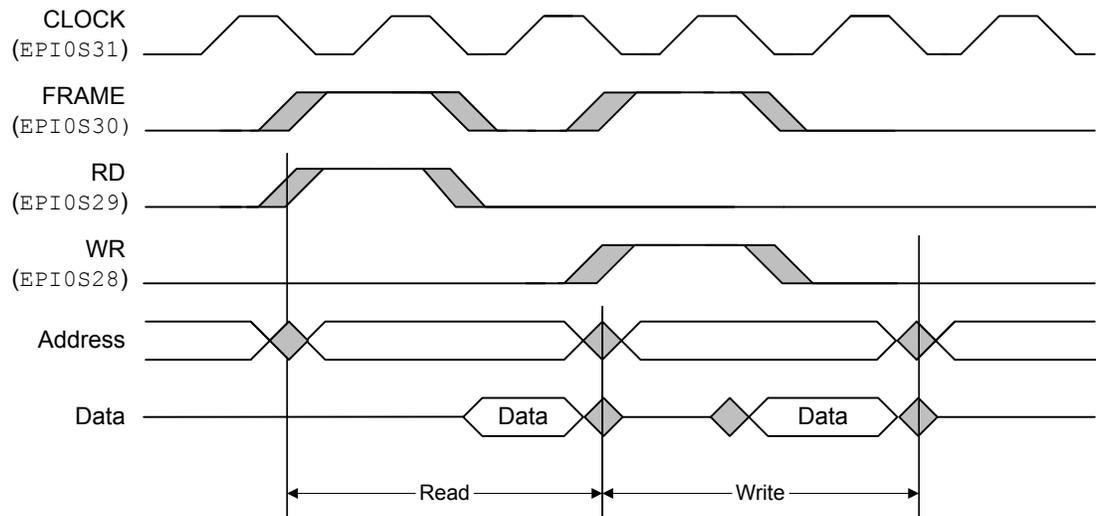
**Figure 11-21. Read Accesses, FRM50=0, FRMCNT=0**
