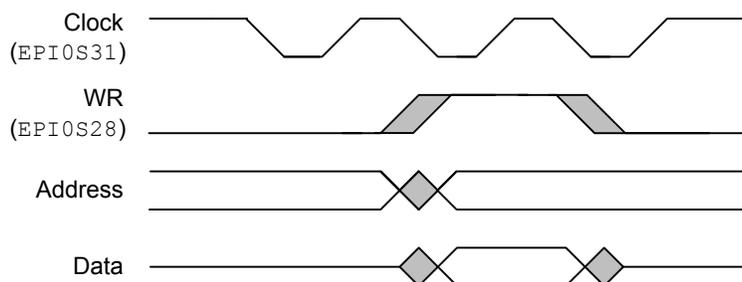
Figure 11-29. EPI Clock Operation, CLKGATE=1, WR2CYC=1
