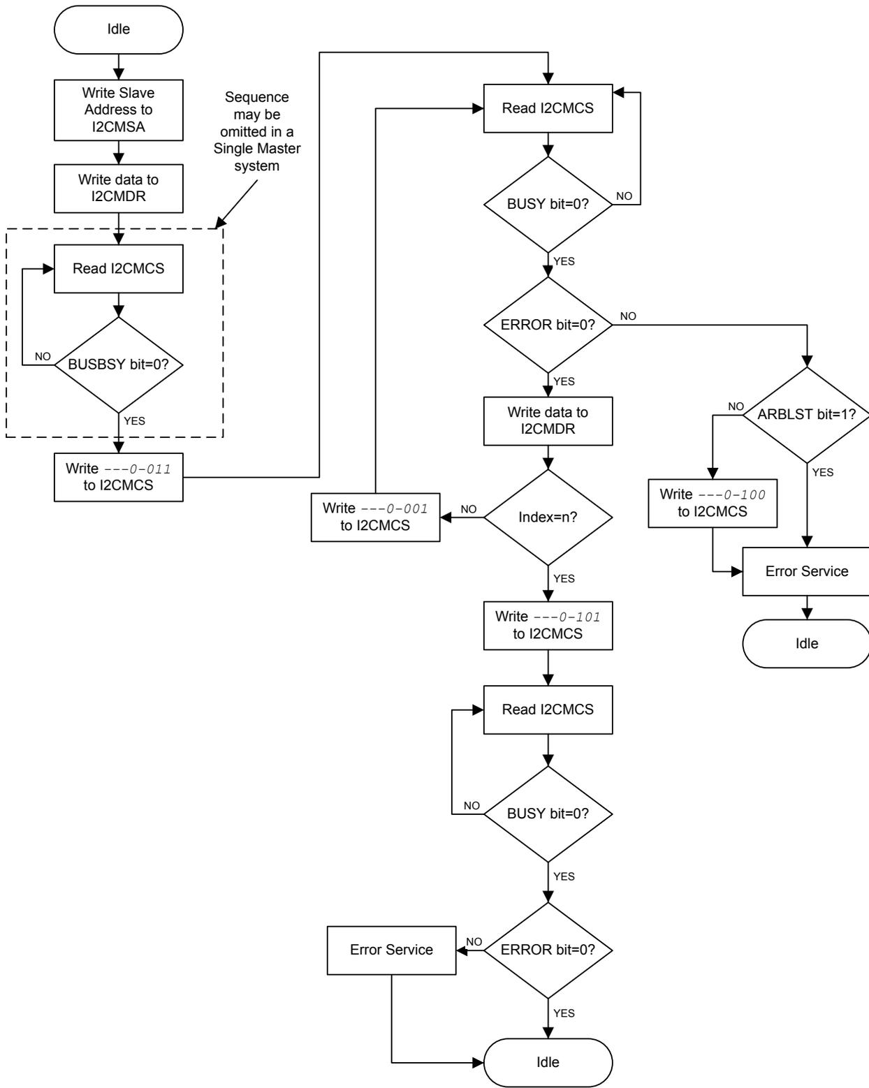
Figure 18-11. Master RECEIVE of Multiple Data Bytes
