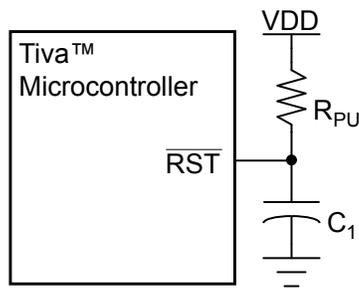
Note:  $R_{PU} = 1$  k $\Omega$  to 100 k $\Omega$
