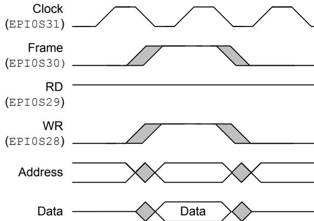
**Figure 11-20. Two-Cycle Read, Write Accesses, FRM50=0, FRMCNT=0, WR2CYC=1**
