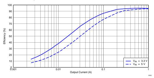
Figure 2. TPS54519EVM-037 Low Current Efficiency
