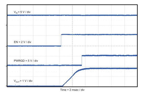
Figure 10. TPS54519EVM-037 Start-Up Relative to Enable
