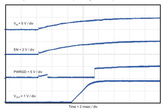
Figure 9. TPS54519EVM-037 Start-Up Relative to V<sub>IN</sub>
