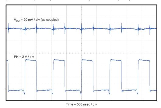
Figure 7. TPS54519EVM-037 Output Ripple
