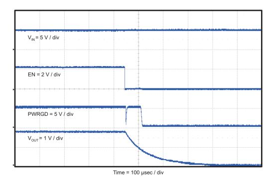
Figure 12. TPS54519EVM-037 Shutdown Relative to EN
