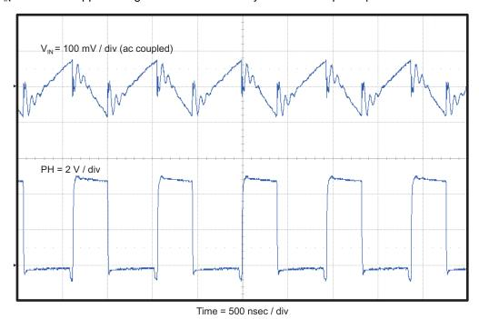
Figure 8. TPS54519EVM-037 Input Ripple
