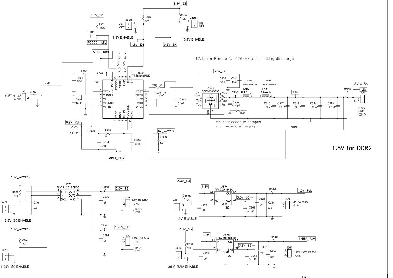
R39x and all connectors / headers are Test Interface Parts
