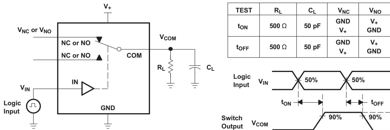
Figure 12. Turnon (t<sub>ON</sub>) and Turnoff (t<sub>OFF</sub>) Time
