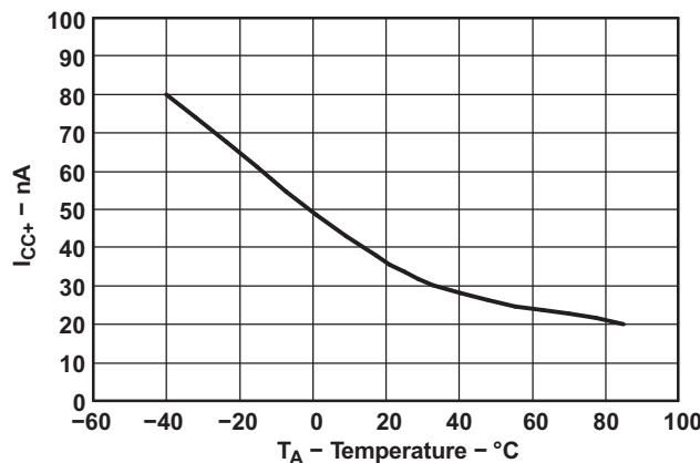
Figure 20. Power-Supply Current vs Temperature ( $V_+ = 5$  V)
