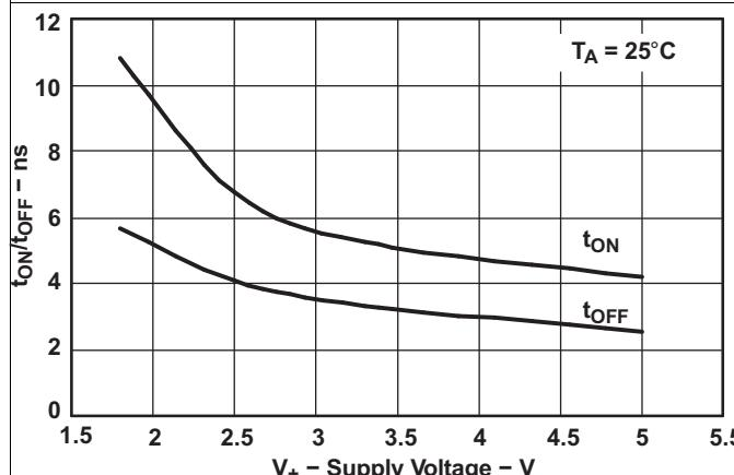
Figure 5.  $t_{ON}$  and  $t_{OFF}$  vs  $V_+$
