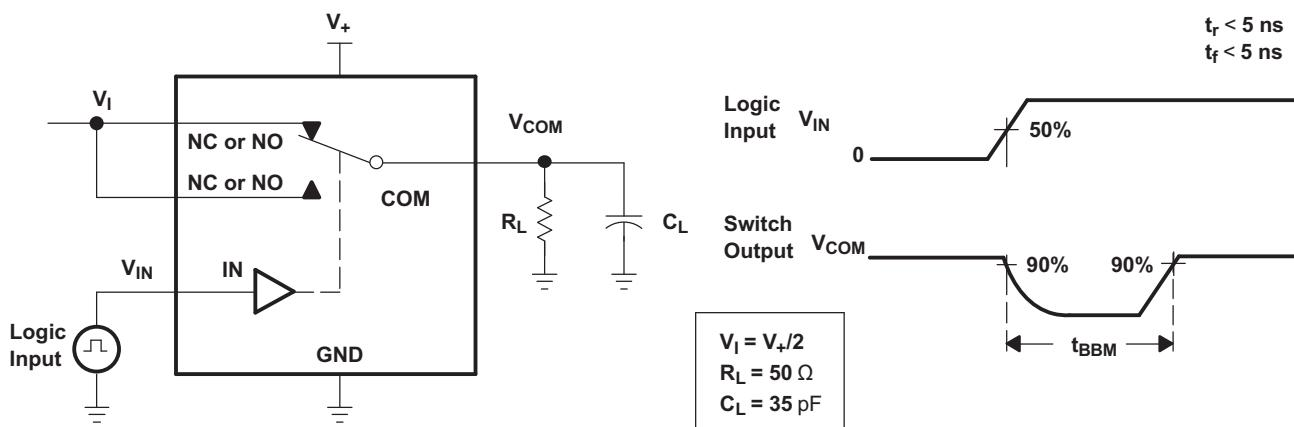
Figure 13. Break-Before-Make (t<sub>BBM</sub>) Time
