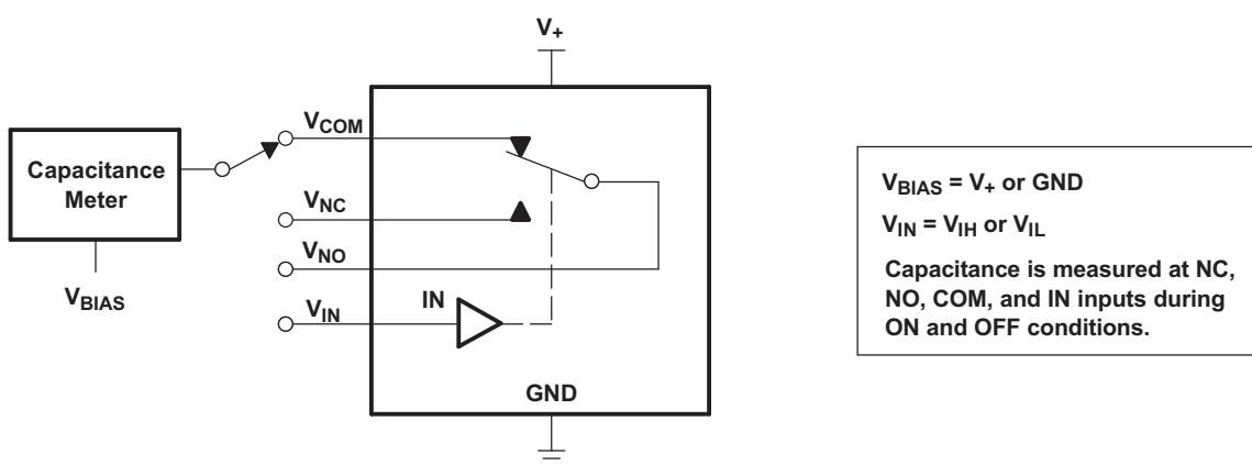
Figure 11. Capacitance ( $C_{IN}$ ,  $C_{COM(ON)}$ ,  $C_{NO(ON)}$ ,  $C_{NO(OFF)}$ ,  $C_{NO(OFF)}$ ,  $C_{NO(ON)}$ )
