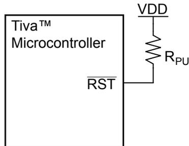
$R_{\text{PU}} = 0$  to 100 k $\Omega$
