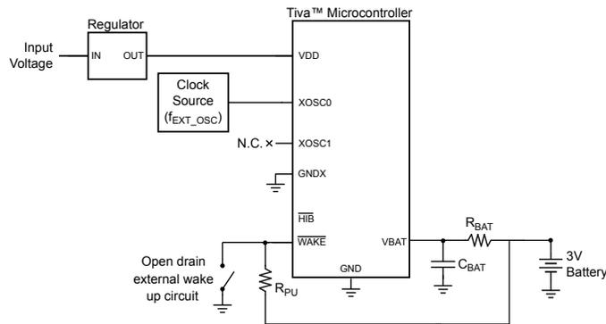
**Note:** Some devices may not supply the GNDX,  $\overline{\text{WAKE}}$  or  $\overline{\text{HIB}}$  signals. See “Signal Tables” on page 1201 for pins specific to your device.
