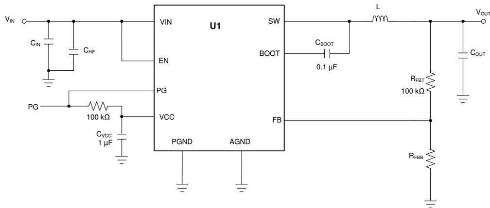
图 8-29. Circuit for Application Curves
