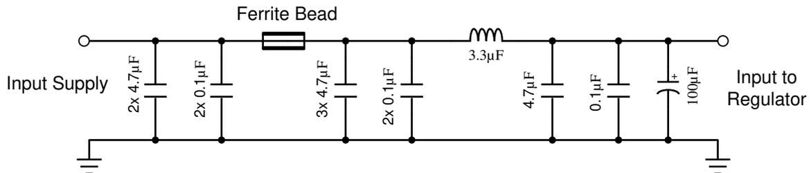
图 8-30. Typical Input EMI Filter
