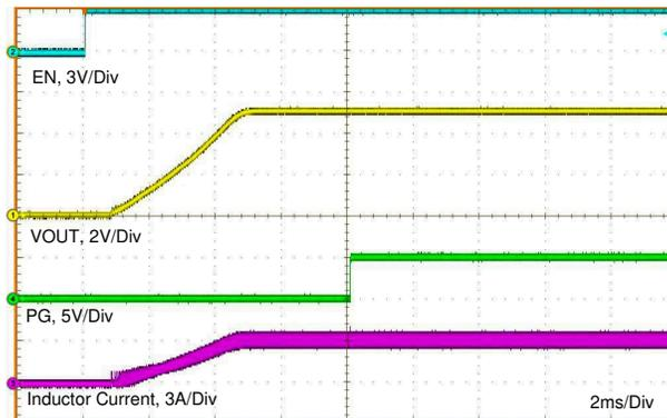
图 7-4. Typical Start-up Behavior  $V_{IN} = 12\text{ V}$ ,  $V_{OUT} = 5\text{ V}$ ,  $I_{OUT} = 3\text{ A}$
