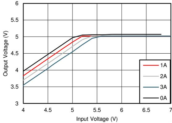
7-9. Overall Dropout Characteristic  $V_{OUT} = 5\text{ V}$
