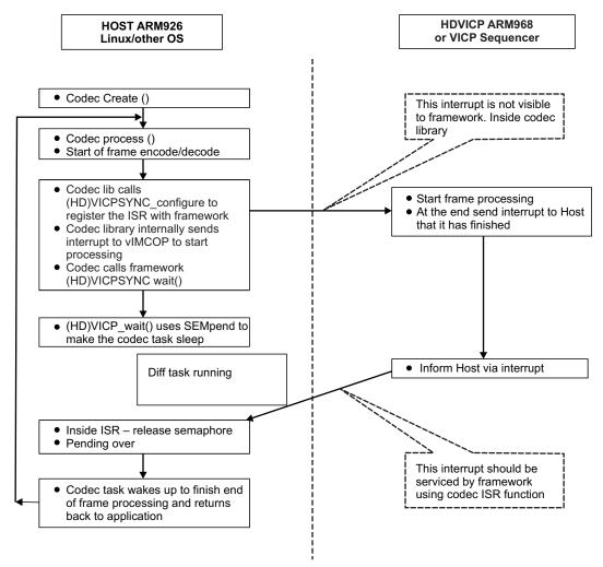
Figure 2. DM365 Codec Architecture, Host  $\leftarrow \rightarrow$  Co-Processor Communication
