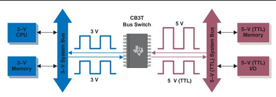
Figure 9. CB3T Device Used to Interface a 3-V Bus With a 5-V (TTL) Bus
