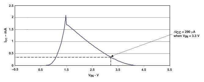
Figure 17. VIN vs ICC Characteristics of SN74HCT541
