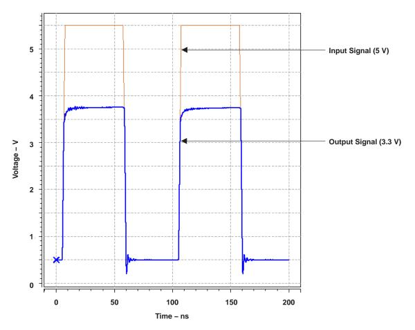
Figure 11. 5-V to 3.3-V Translation Using CBT Device
