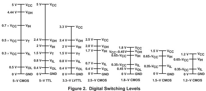
Figure 2. Digital Switching Leve
