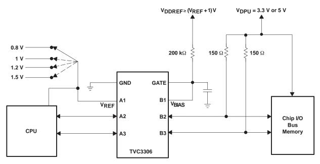
Figure 13. SN74TVC3306 Used in a Level-Translation Application
