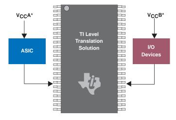
\*V<sub>CC</sub>A not equal to V<sub>CC</sub>B
