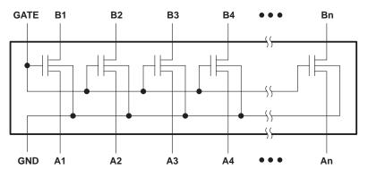
Figure 12. Simplified Schematic of a Typical TVC-Family Device
