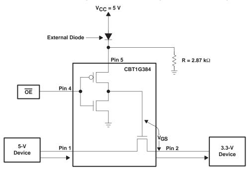
Figure 10. SN74CBT1G384 In 5-V to 3.3-V Application
