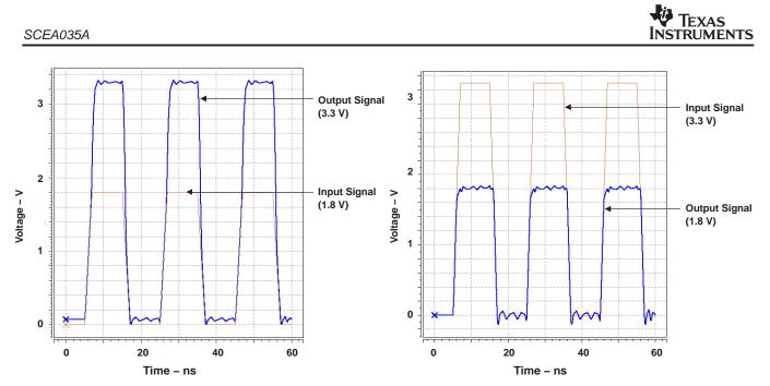
Figure 14. Waveforms For Bidirectional Translation Using a TVC Device
