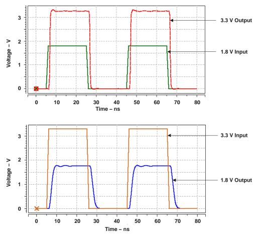
Figure 3. SN74AVCB324245 Translating From 1.8 V to 3.3 V (Bank 1) and 3.3 V to 1.8 V (Bank 2) at the Same Time (C<sub>L</sub> = 15 pF, R<sub>L</sub> = 2 k $\Omega$ )
