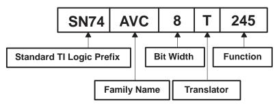
Figure 4. Dual-Supply Level-Translation Device Nomenclature
